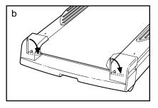
the treadmill for a few minutes. Repeat until the walking belt is properly tightened.
